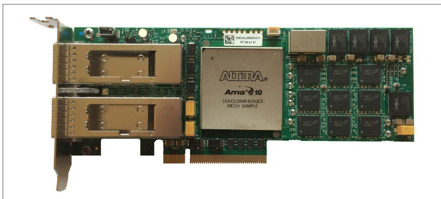
Figure 2 | BittWare's A10PL4 low-profile PCIe board is based on Altera's Arria 10 FPGA, and includes 8x 10 GbE, 2x 40 GbE, or 2x 100 GbE network interfaces and up to 32 gigabytes of DDR4.
